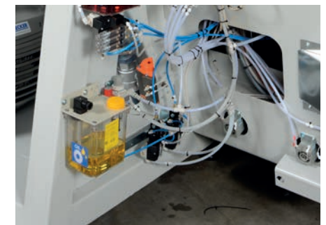
Automatic lubrication for tools
