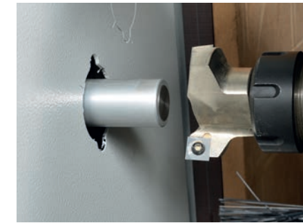
Automatic presetter for tool length
