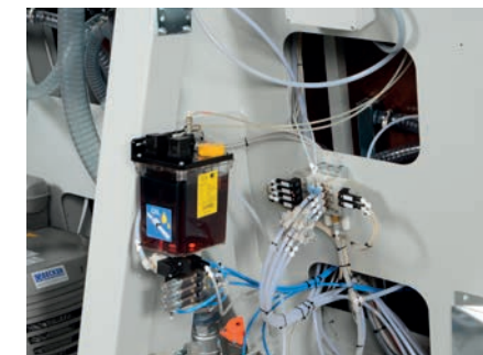
Automatic lubrication for linear guides
