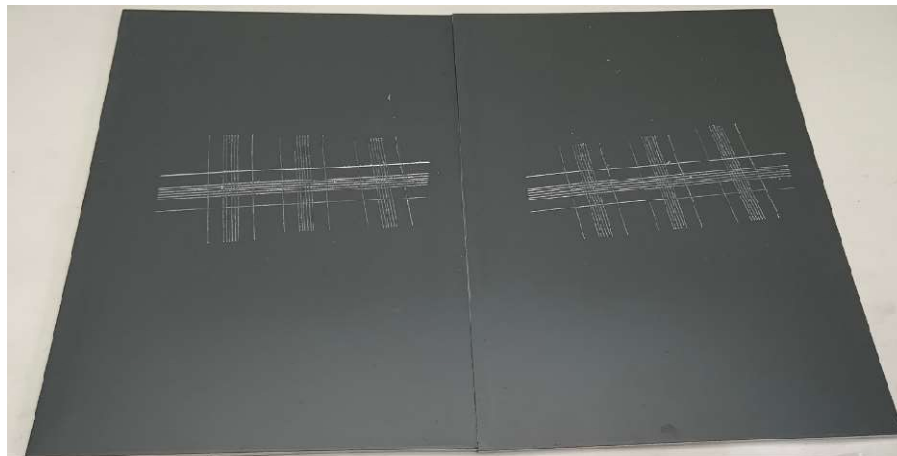
Figure 6 - Wet Adhesion Panels 7 & 8
