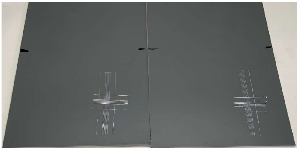
Figure 12 - Detergent Resistance Panels 18 & 19
