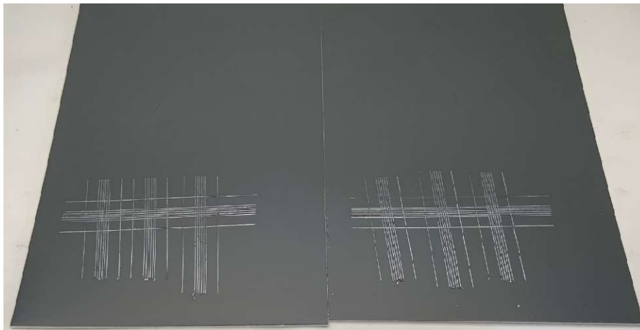
Figure 4 - Dry Adhesion Panels 11 & 12
