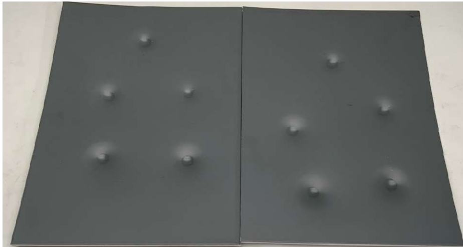
Figure 7 - Impact Resistance Panels 13 & 14
