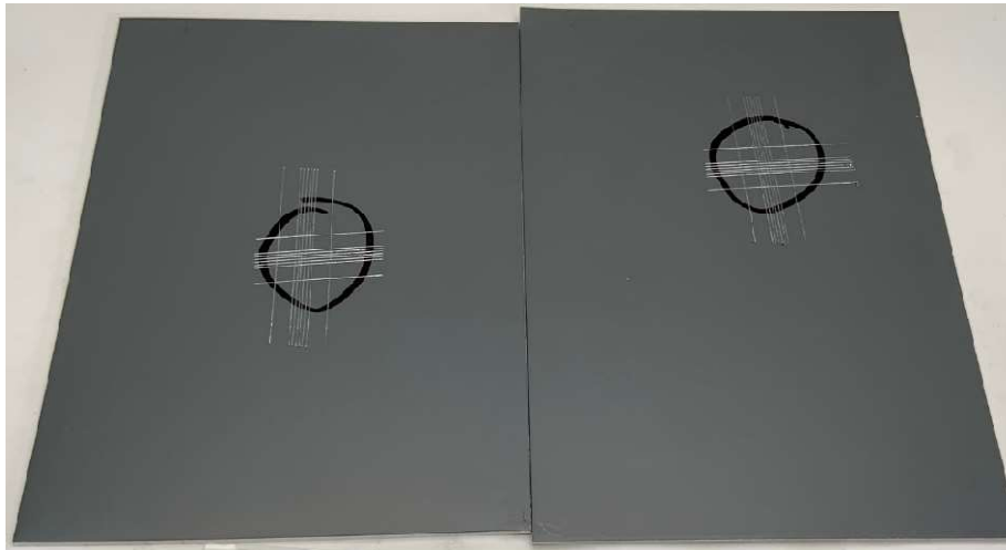
Figure 13 - Window Cleaner Resistance Panels 22 & 23
