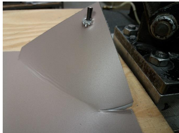
Plate 5.5.2: Example of pull through using a rivet in the corner position (post-test).
