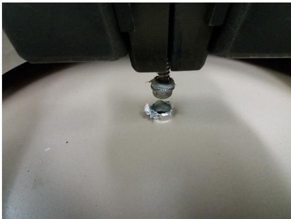
Plate 5.5.1: Example of pull through using a screw in the centre position (post-test).
